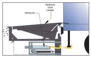
**Benefits:** The "under dock" position of the restraint protects the restraint from adverse conditions on the outside of the dock area. Only the restraint arm is exposed to the external adverse elements at the loading dock. The concerns highlighted below are eliminated.
