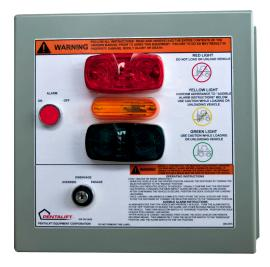
NEMA 12 interior wall mount control station. High visibility interior signal lights are coordinated with exterior signal lights. Clear, concise and easy to follow instructions guide dock attendant on how to use the system. Selector switch and amber light accommodate "override" mode. CSA certified for the design and manufacture of industrial control equipment.
