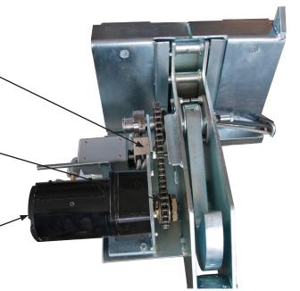
Note: Vehicle restraint is shown with gearbox cover removed to expose components (listed above) that are normally protected by heavy duty cover.
