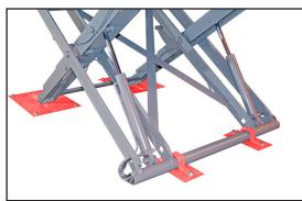
Optional retaining cradles and wear plates (shown in red to accommodate easier visualization) are a recommended option This option also increases the end edge load rating of the lift Lift cams and cylinders translate to full use of deck plate surface, without obstructions
