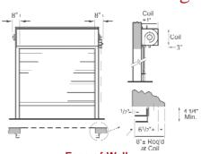
Face of Wall Maintains clearance of full opening, minimal exposed components.
