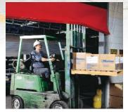
Matadoor® A highly visible safety orange colored breakaway curtain bottom section that controls damage and opening downtime.
