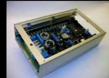
Eight standard inputs, two standard outputs and six additional field programmable I/O's
