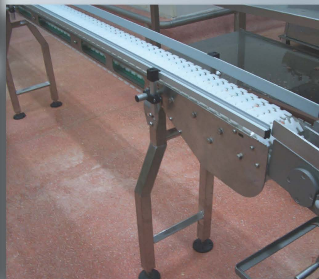
Rigid support structure with easy cleaning design.
