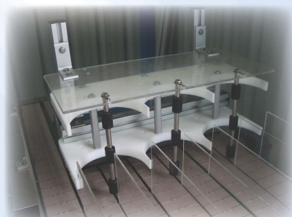
To avoid can from toppled when transferring from one conveyor line to another
