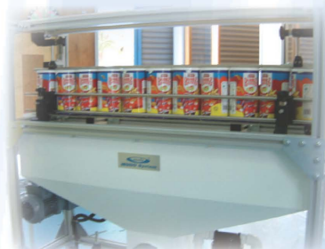
Product is transported to another machine while being dust blowing.
